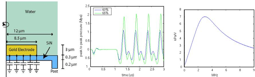
**FIGURE 5.** A dual-mode endoscopic CMUT transducer was modeled in ANSYS (left). A maximum output pressure was calculated to be in excess of 2 MPa peak-to-peak at 2 MHz (center). With a bandwidth of ~90% and the sensitivity 7.5kPa/V, the transducer can image at 3 MHz (right).
