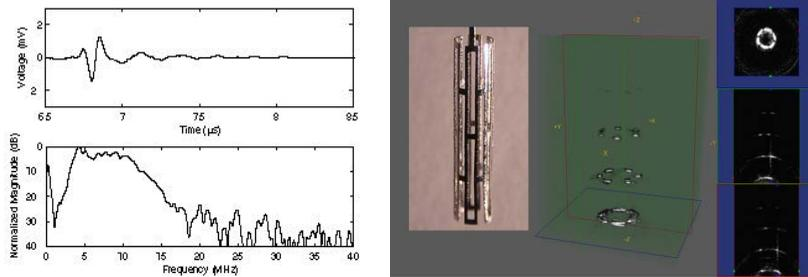
**FIGURE 3.** Typical pulse-echo response and frequency response of the CMUT ring array (left). 3-D image (right) of a stent taken by the 64-element annular ring array; a picture of the stent is shown on the left for comparison [11].
