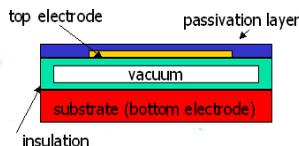
**FIGURE 1.** A simplified cross-section of a CMUT.
