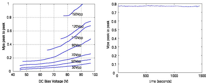
**FIGURE 4.** A wafer-bonded device has been demonstrated to produce output pressures as high as 1 MPa (left). The device also achieved 0.7 MPa peak-to-peak consistently in continuous wave mode with 80 V bias voltage and 130 Vpp AC voltage (right). The slight decrease in output pressure with time is probably caused by oxide charging.
