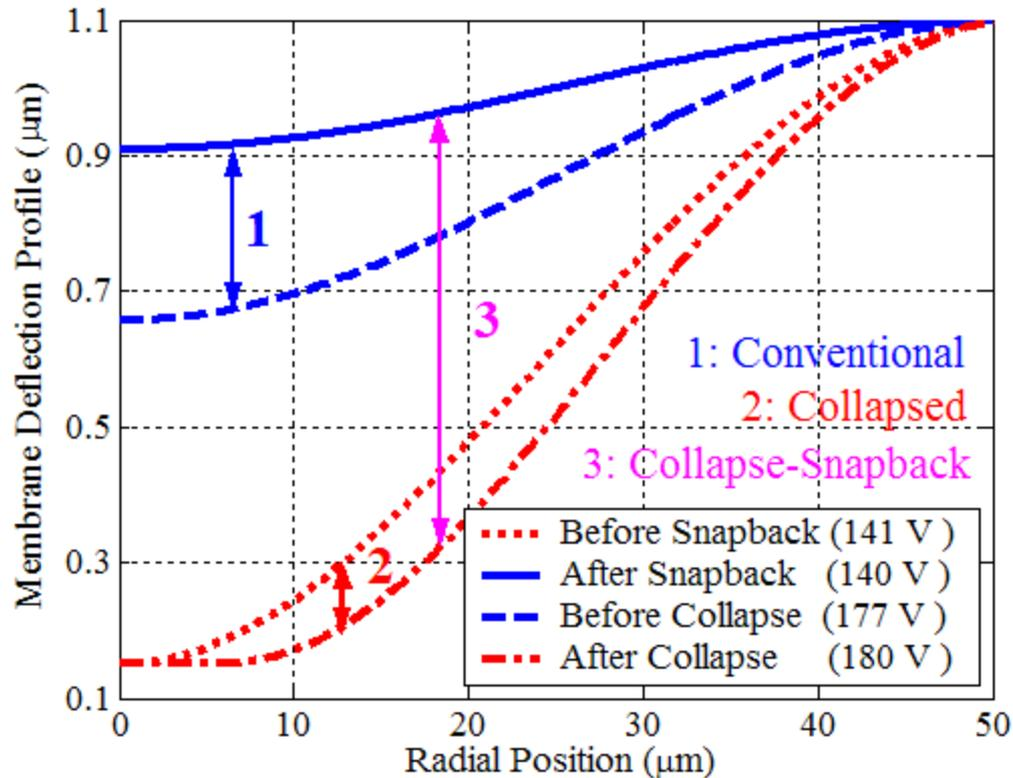
Conventional, Collapsed and Collapse-Snapback Operations
